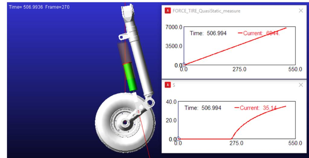
Figure: Landing gear quasi-static test
