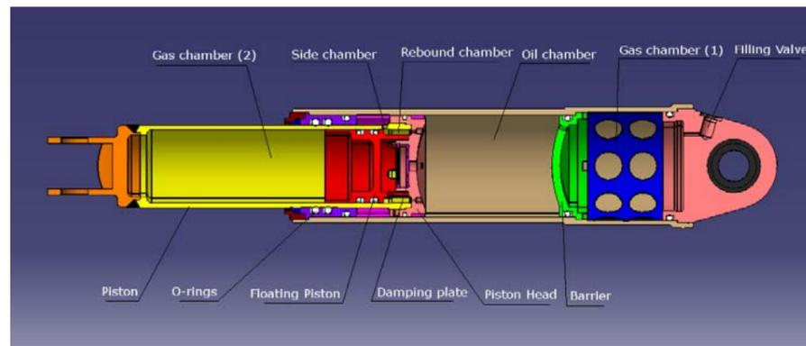
Figure: Shock absorber cross section
