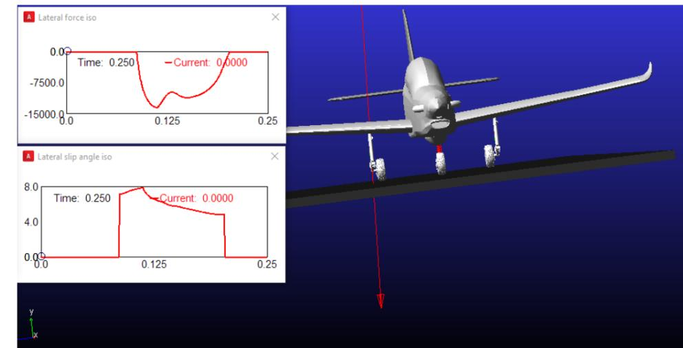
Figure: Complete aircraft model in MSC.ADAMS
